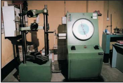
Universal Testing Machine 60 tonnes for testing of hoop tensile and axile tensile of pipes
